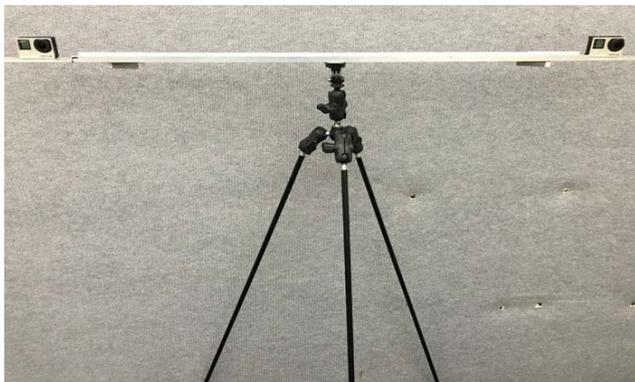
**FIGURE 1.** Stereo camera rig on a tripod with a baseline distance of one meter.
